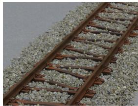
With the point contacts etched from nickel silver sheet metal can many 2L flex tracks be converted to 3L flex track. The best result will be reached with Weinert sleeper gratings, Code 83 profiles from Tillig (burnished) and our point contacts. Why not Tillig Elite Flextrack? Tillig has on both sides of the profiles the screws imitated, the high 3L Wheel flanges would run up. Also is the soft plastic from Tillig not optimal suitable for retrofitting.
